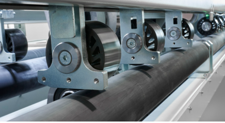
Transport- and pressure rollers with automatic height adjustment Positioning format specific and according to FEFCO-type
